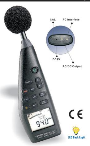
Our advanced sound level meter CENTER 390 fully complies with IEC61672-1. This meter has only one measuring range and it is extending from 30db to 130db, which is full 100db. The operator will not have to worry about which range to use like in the 3 or 4 range models and neither about signal latency in auto range models. This unit is also a data logger and it is equipped with manual storing capability which can store 99 sets of data and can be readout from the unit or through PC.
