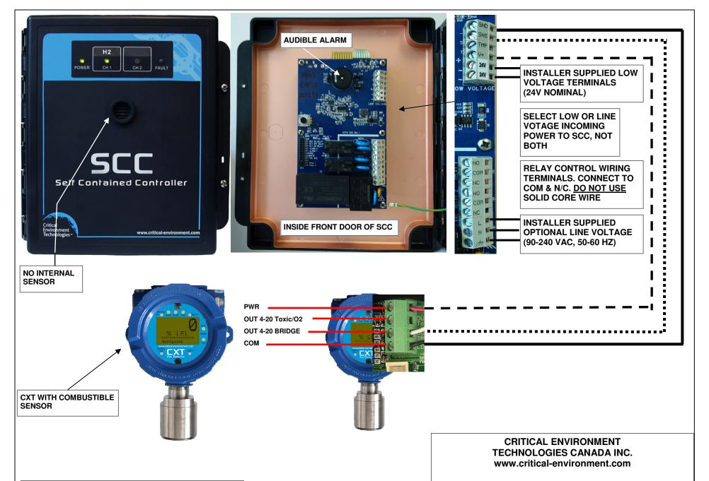
THIS SCC-B-RT WITH CXT COMBUSTIBLE COMBINATION MAKES A ONE CHANNEL DETECTION SYSTEM.
