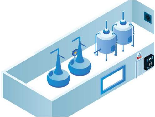
than air and will accumulate in enclosed areas, low lying areas and downstream from the vapour source. It should be installed near the most likely potential area of exposure.
