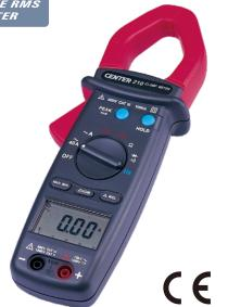
CENTER 210 series are mid-size clamp meters. These clamps can measure up to 1000A with resolution 0.01A. 1 ms peak function is also built-in this series of clamps. This is especially useful for start current measurement. Maximum, Minimum and Hold are also standard functions for these testers.
