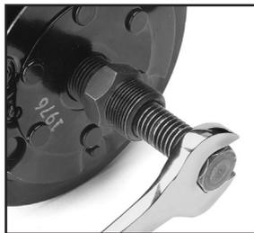
Tech Tip: Proper air gap between the clutch pulley and hub armature is critical to compressor overall performance. Failure to maintain the proper spacing, as indicated in the mfgs. specifications can lead to problems such as clutch burning or slippage.
