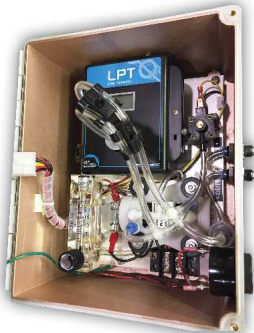
Inside of the DCC-SD showing an LPT-A gas detector mounted inside the enclosure.
