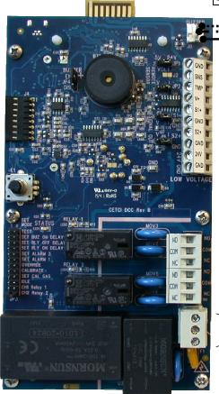
LINE VOLTAGE WIRING TERMINAL 90—240VAC **NOTE:** Two SPDT dry contact relays, including VFD control, rated 5 amps @ 240 VAC RELAYS OPERATE IN FAIL SAFE CONFIGURATION.
