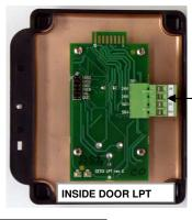
LPT 2-WIRE ANALOG TRANSMITTER WIRED TO DCC DUAL CHANNEL CONTROLLER
