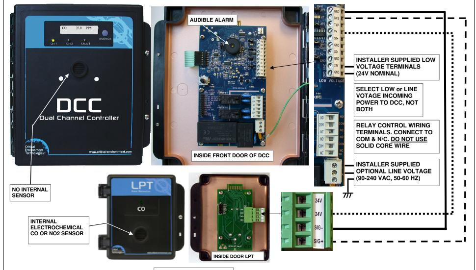
LPT 3-WIRE ANALOG TRANSMITTER WIRED TO DCC DUAL CHANNEL CONTROLLER
