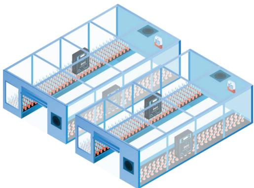
will monitor approximately 650 sq m (7,000 sq ft). The most appropriate location for the device to be installed is close to where people frequent the most such as pathways and work areas inside the growing area.
