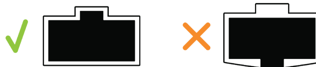
Figure 3-5 - Ribbon Cable Orientation
