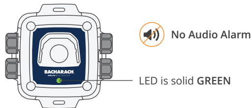
Figure 4-3 - Inspecting Connected MGS-410
