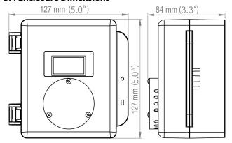
Above dimensions are shown with optional splash guard. Without splash guard, thickness is  $71 \, \text{mm} / 2.8 \, \text{in}$ . The area required for enclosure door to be open 90 degrees is  $178 \, \text{mm} / 7.0 \, \text{in}$  or  $254 \, \text{mm} / 10.0 \, \text{in}$  for fully open. With the optional splash guard installed, the enclosure is IP54 rated.
