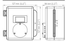
Note: Drawings above are shown with the optional splash quard. Without the splash guard, the thickness of the unit is 71 mm (2.8").
