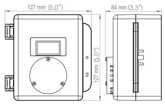
Above dimensions are shown with optional splash guard. Without splash guard, thickness is 71 mm (2.8"). The area required for enclosure door to be open 90 degrees is 178 mm (7.0") or 254 mm (10.0") for fully open. With the optional splash guard installed, the enclosure is IP54 rated.
