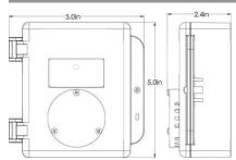
Note: Drawings above are shown with an optional splash guard. Without splash guard, thickness of unit is 53.34 mm (2.1 inches).
