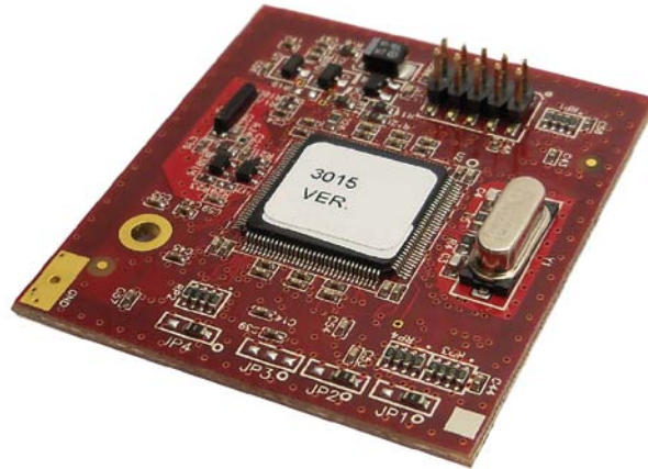
Figure 4. Microprocessor Module Removed from PAGM Main Board
